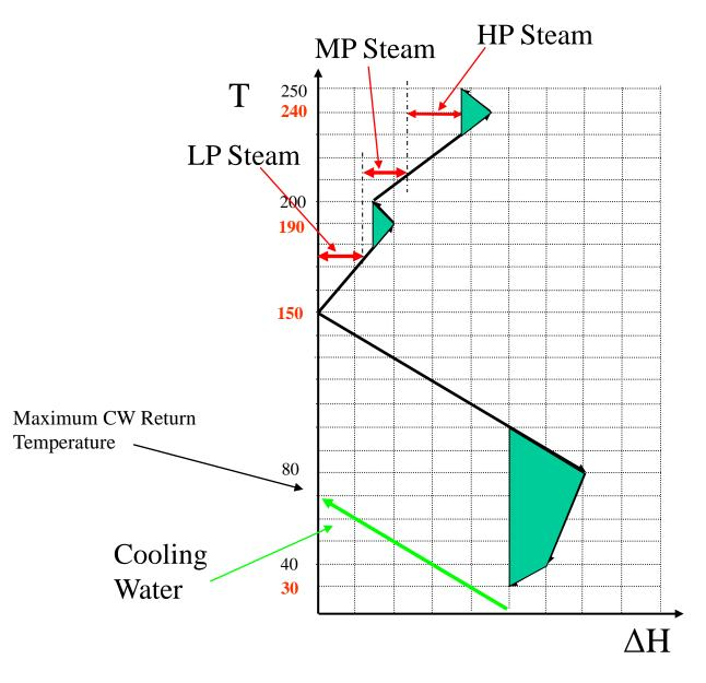
Cooling Water line should not cross the Grand Composite Curve
